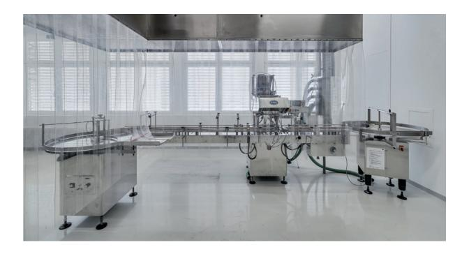
This machine is used to package tablets, capsules and dragées fully automatically in jars.
