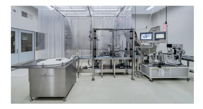
This machine is used to package solids fully automatically in screw-top or cardboard jars.
